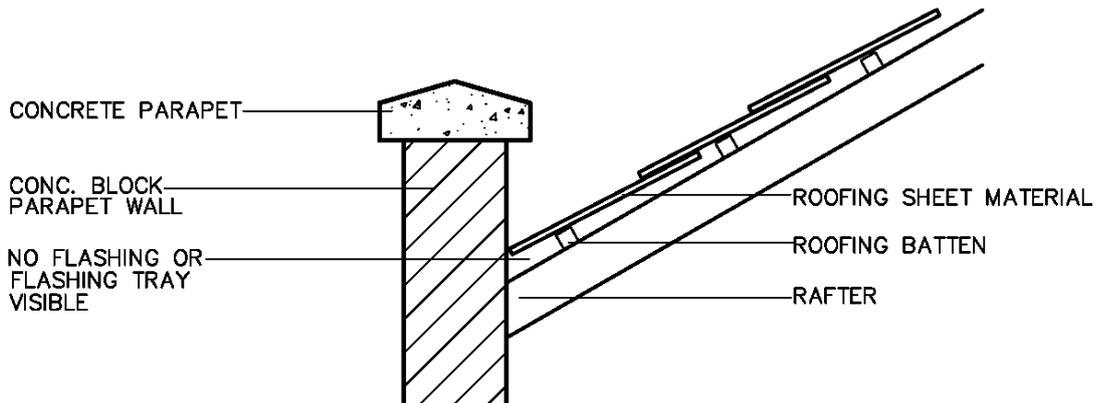
**PARAPET DETAIL (N.T.S.) (as visible on site)**
