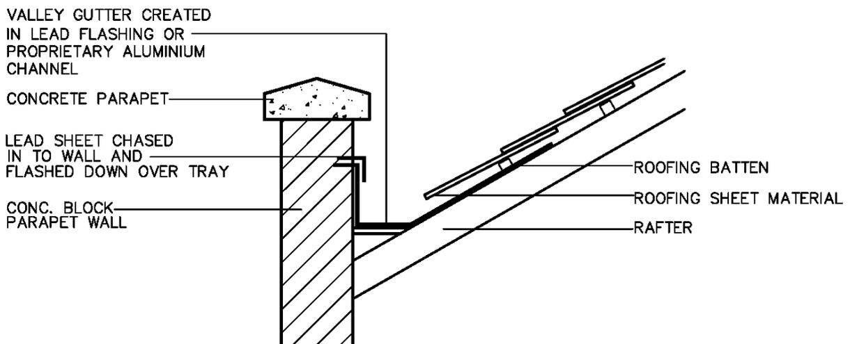
**CORRECT PARAPET DETAIL (N.T.S.)**
